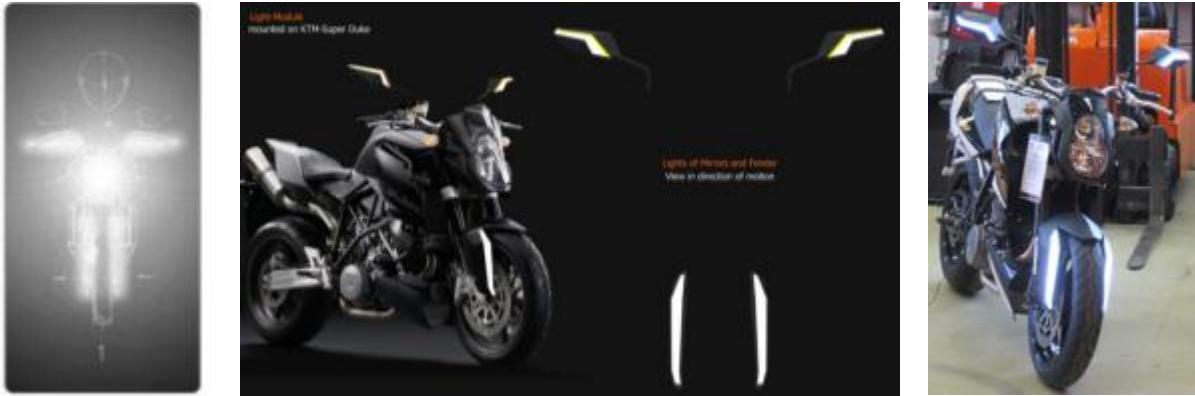
Figure 57: Alternative Front Light Patterns; T-light configuration
