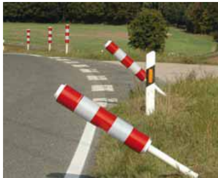
Figure 18: Guide posts made of flexible material 17
