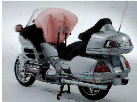
Figure 35: Honda's motorcycle airbag system 31
