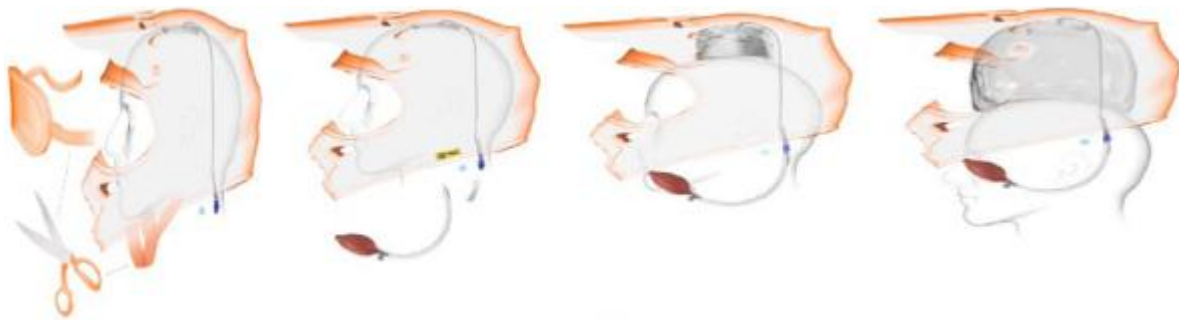
Figure 87: Eject Helmet Removal System Procedure 82
