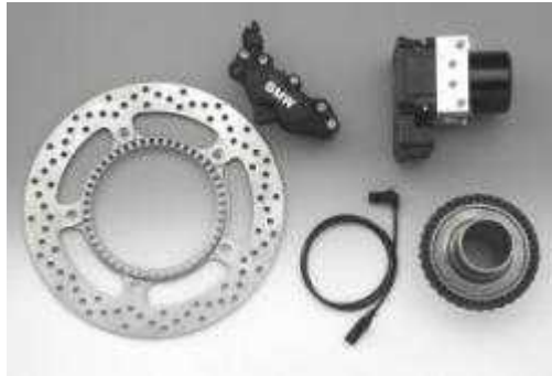
Figure 33: BMW, elements of an ASC systems
