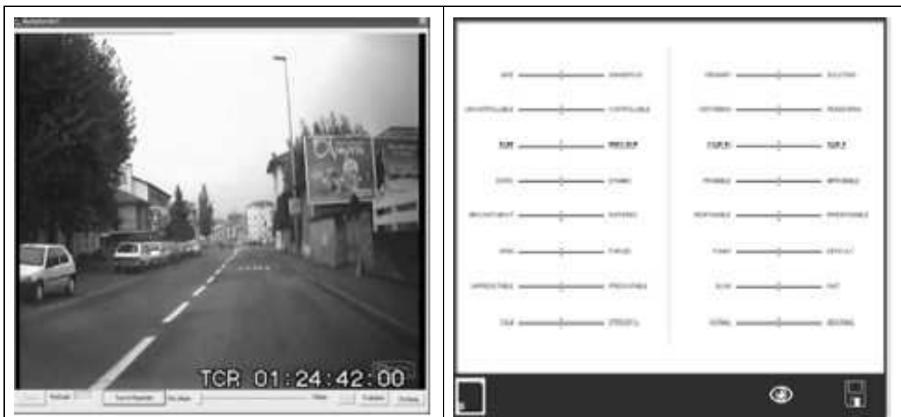
Figure 10: CRITIC: a methodological tool for studying drivers' risk awareness abilities, including a Likert Scale (on the left, below the road scene view) and an Osgood Semantic Differential (on the right); Banet and Bellet, 2008)
